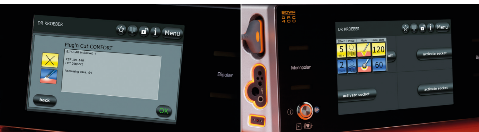
Plug'n Cut COMFORT: The COMFORT SYSTEM automatically recognises the COMFORT instrument, indicates how many times it may still be used and selects the correct parameters for the procedure
