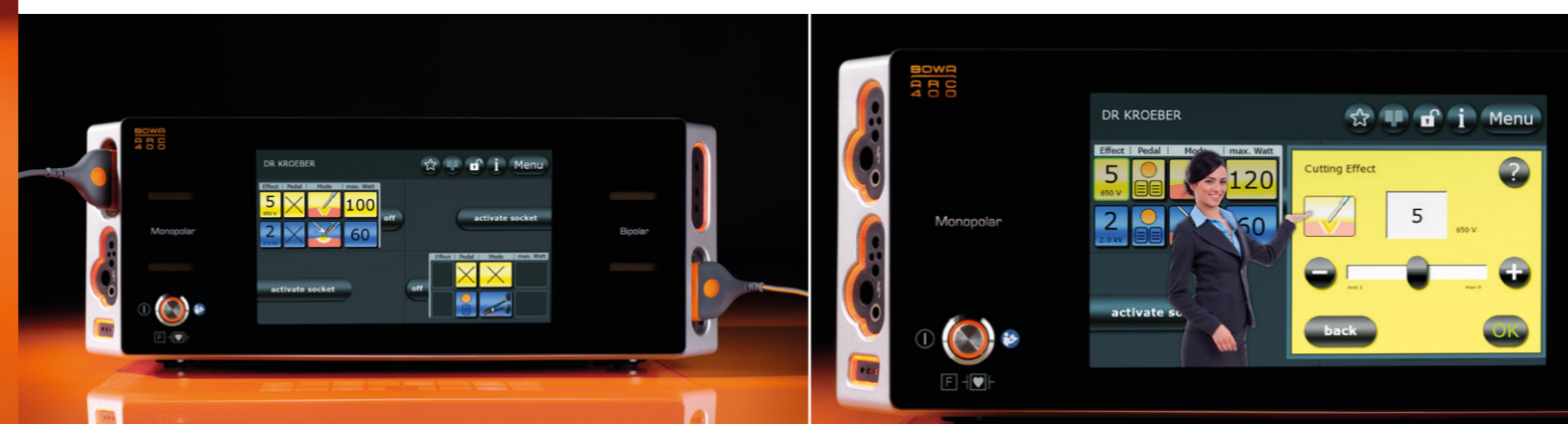
Clarity: Every connected socket – in this photo the upper left and lower right – is clearly assigned to one quadrant of the display
