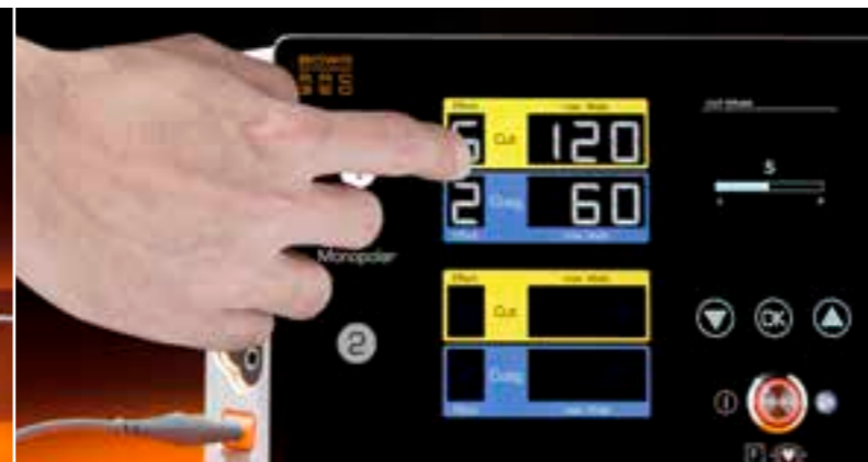
Simple to use: Tap the corresponding field to activate the input menu in the centre of the ARC 350 to adjust effects or power values
